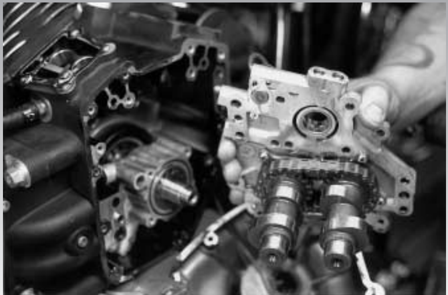
Remove and replace cams
